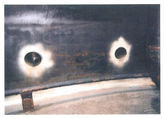
Bottom corner weld MPI 100% of cir. All nozzle penetrations MPI 100%
